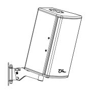
If further pan and tilt adjustment is necessary remove the cabinet from the bracket before loosening any adjustment nuts. NEVER adjust with the cabinet on the bracket.
