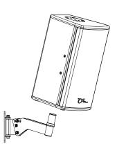
When all mounting and adjusting hardware has been fully tightened, present the cabinet to the bracket. Ease the cabinet onto the mounting pole.
